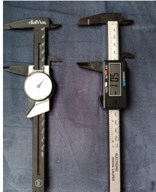
Figure 8; The mechanical and the digital calliper. Both give an accuracy of 10^{-4} cm.
